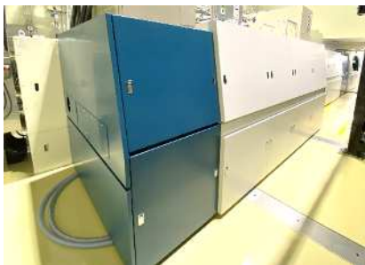
Fig.1 LD pumped 250 J Yb:YAG ceramics laser.
